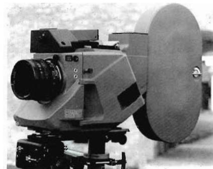
COMPACT on Steadicam. Magazine is prototype fabricated from Arri IIC mag. Made out of Kevlar, the final design will be lighter, sleeker, and closer to camera body.
