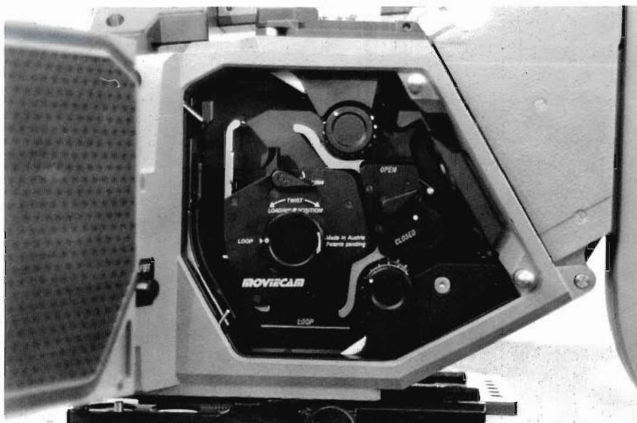
COMPACT movement permits very fast threading. Knobs are pushed in to quickly adjust loop
