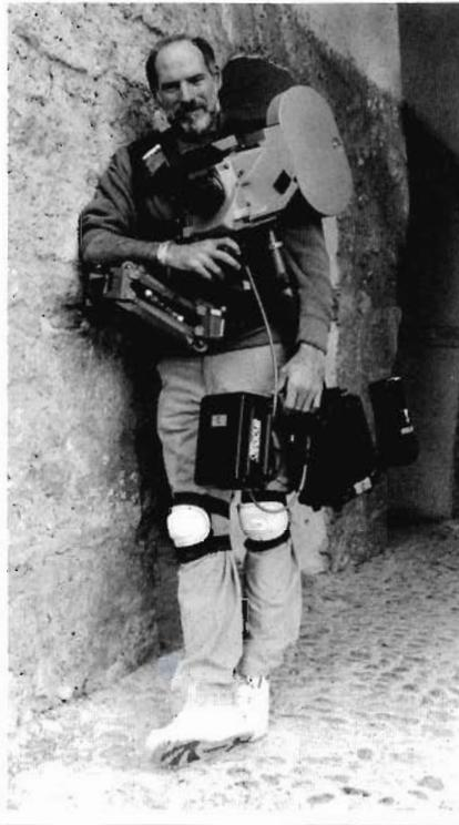
Churchill with Moviecam Compact at Steadicam class outside Munich, Germany last fall. The camera feels wonderful on the Steadicam because most of the weight is concentrated directly over the center post
