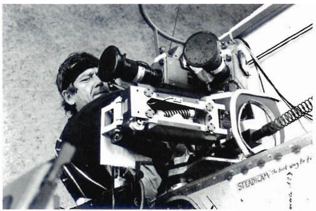
The three cameras and part of the Bringuier-Wuthrich system. Notice the zooms of the Betas are locked to 30° with metal pieces. Also note: "Steadicam..."
